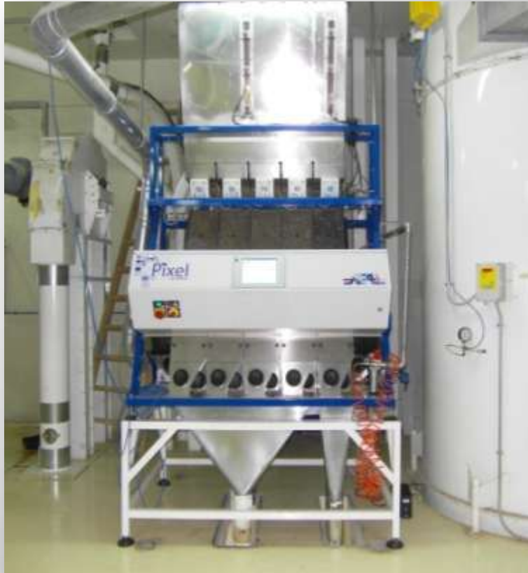
STANDARD INSTALLATION WITH LOADING & DISCHARGING HOPPERS AND SUPPORTING FRAME
