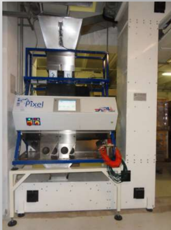
EXAMPLE OF INSTALLATION WITH ELEVATOR.
